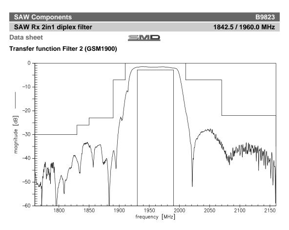
Transfer function Filter 2 (GSM1900) - Wideband
