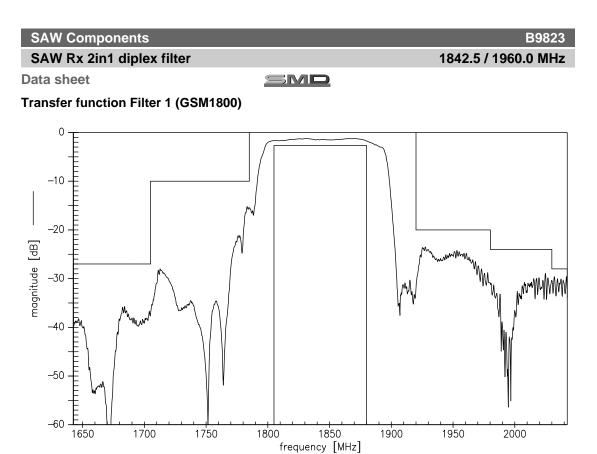
Transfer function Filter 1 (GSM1800) - Wideband
